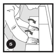
Press tiles firmly against adjoining tiles and lay row by row or in a pyramid fashion. Press firmly into adhesives.
