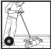
Roll entire installation with a minimum of 100-pound floor roller.
