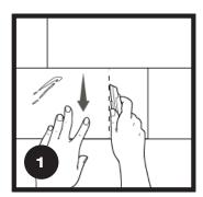
Using a utility knife, cut a seam lengthwise through the damaged plank.
