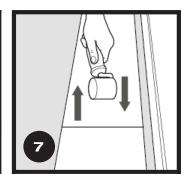
Use a resilient flooring hand roller to squeeze out any remaining adhesive in tight spaces.
