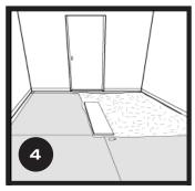
After sufficient open time, begin laying the tile from the center point, making sure the tile is squarely on the lines.
