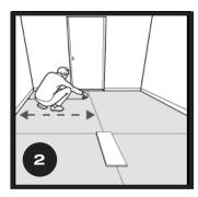
Measure the distance from the center to the wall. Divide the measurement by the width of the plank. If less than half the width remains as the border plank, adjust the center point by half the width of a plank.
