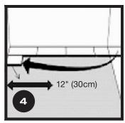
Start the second row with the leftover cut part of the last plank of the previous row. This small plank should measure at least 12" (30cm). Otherwise, cut a new plank in half and use it to begin the second row. Whenever practical, use the piece cut from the preceding row to start the next row.
