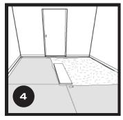
After sufficient open time, begin laying the tile from the center point, making sure the tile is squarely on the lines.
