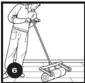
Roll entire installation with a minimum of 100-pound floor roller.
