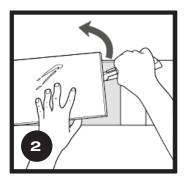
Insert a thin 2" wide putty knife in the cut line and gently lift up.
